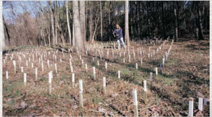
The effectiveness of preservatives at various retentions in different species is evaluated using test stakes.
